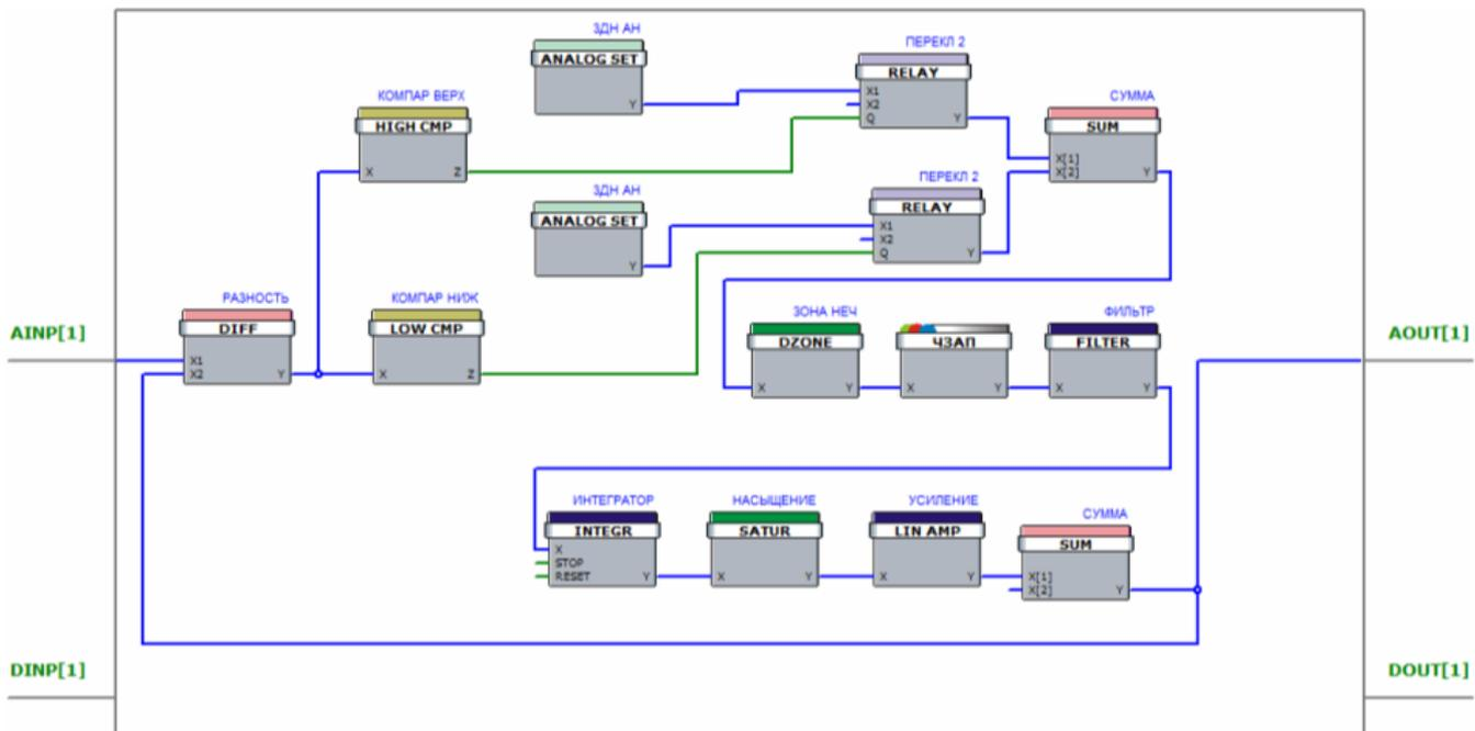
**Fig. 5 – EIM imitating model of proportional action**
