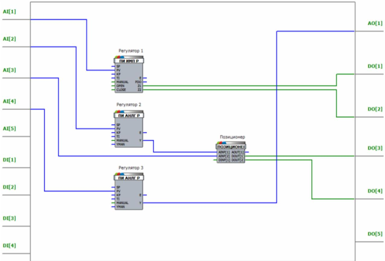
Fig. 2 – Regulating Controller MC5 of the complex “КОНТАР”
