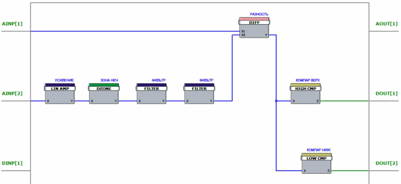
Fig. 3 – Block diagram of a positioner
